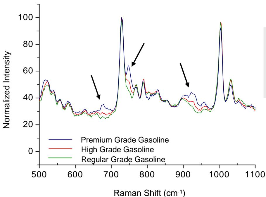
Using the Vector Raman Probe™, quality control of gasoline grades can be achieved, as illustrated in the composite spectra on the left. Compositional changes are observed as grade-specific differences in normalized Raman peak intensities.
