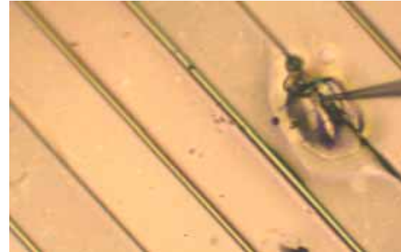
Taking off the part of particle with glass tip
